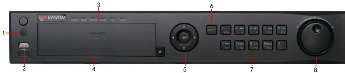
1. **IR Receiver:** operation by IR remote control.
