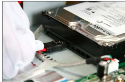
**4.** Connect the power cable to the HDD.
